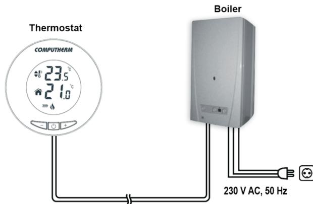
Temperature can be measured and set at digital display more precisely as compared to simple, conventional thermostats. In heating mode, the thermostat switches the boiler or any other appliances on below and off above the adjusted temperature, respectively, and contributes to reduce energy costs while maintaining comfort. In cooling mode it switches the opposite way.
