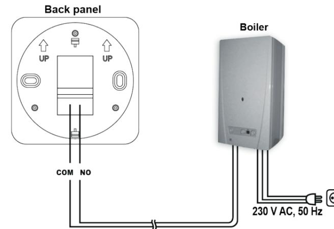
If you would like to operate an old boiler or any other device that has no connection points for thermostats, then the **NO** and **COM** connection points of the thermostat should be connected to the mains cable of the device, similarly as a switch would be connected.
